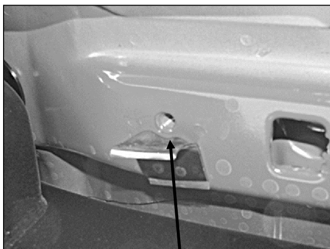
(Fig 5) 8mm threaded hole in "closed" floor frame channel (passenger side-front pictured for example)
