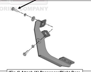
(Fig 4) Attach (1) Passenger/Right Rear **Mounting Bracket to the center location**
