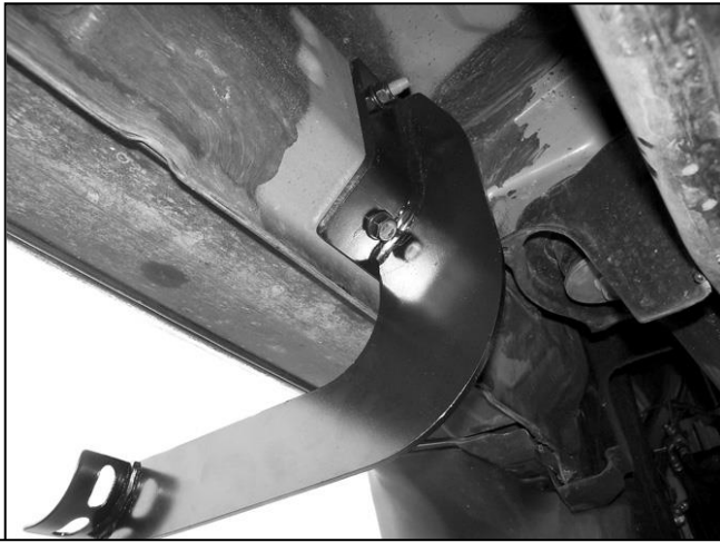
(Fig 3) Up to 2015 Driver side front Bracket installed
