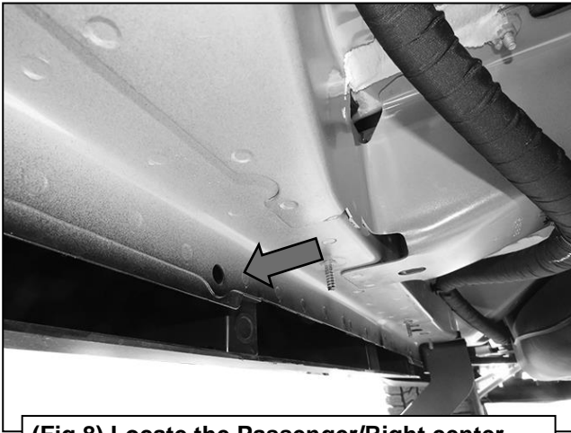
(Fig 8) Locate the Passenger/Right center mounting location. Line up the top of the Passenger/Right Center Mounting Bracket to the hole in the pinch trim. Mark the top slot for drilling. Use a 1/2" drill bit, not included
