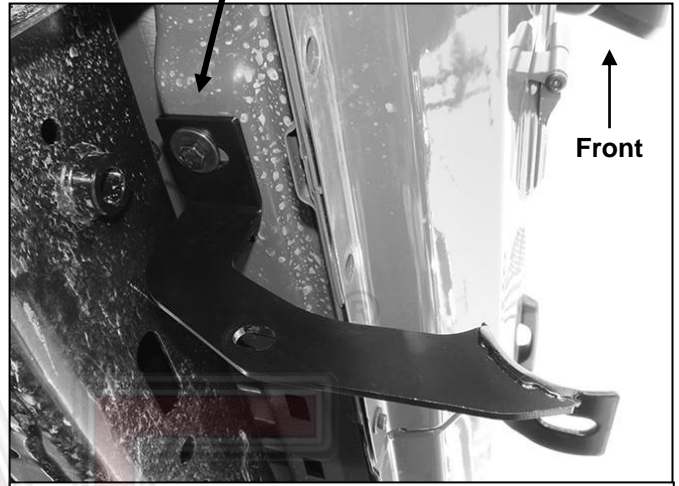
(Fig 4) Driver/left front Mounting Bracket installed
