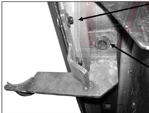
(Fig 3A) Passenger side Front Mounting Bracket installation pictured ("mid length" bracket)
