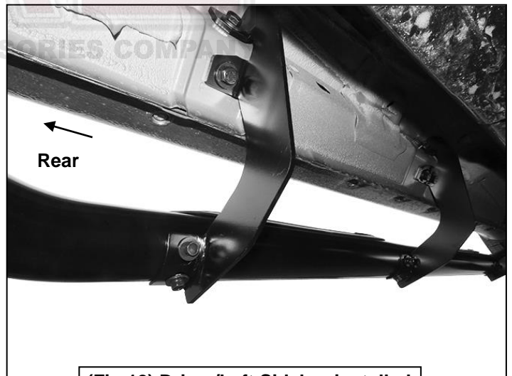
(Fig 12) Driver/Left Sidebar installed on Rear Mounting Bracket
