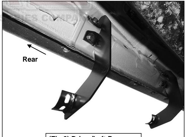
(Fig 8) Driver/Left Rear Mounting Bracket installed
