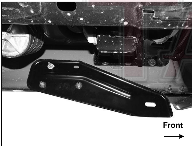
(Fig 3) Driver/left Front Bracket installed
