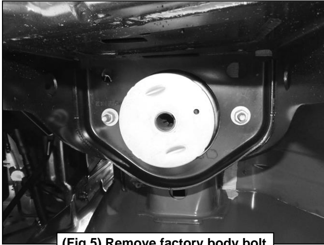
(Fig 5) Remove factory body bolt
