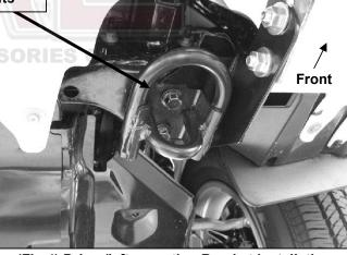
(Fig 4) Driver/left mounting Bracket installation
