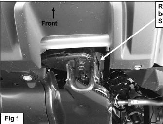
Remove (2) factory hex bolts to remove tow hook. Small tow hook pictured
