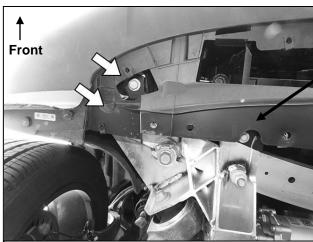
(Fig 1) Remove splash guard. Locate the large 21mm (under plastic cover) and small 16mm (visible) hex bolts (arrows)
