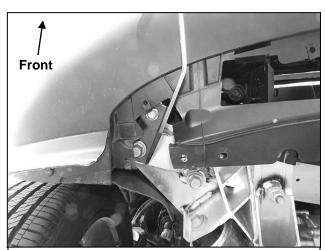
(Fig 4) Slide the inner slot end of the Bracket under the larger 21mm hex bolt. Reuse the 16mm hex bolt to attach Bracket
