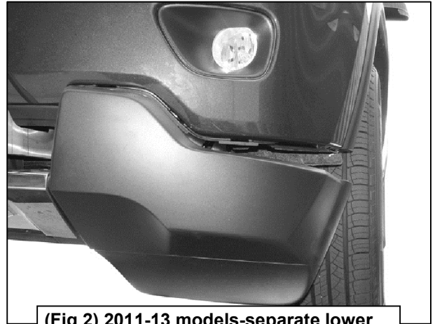
(Fig 2) 2011-13 models-separate lower bumper cover from upper cover at ends
