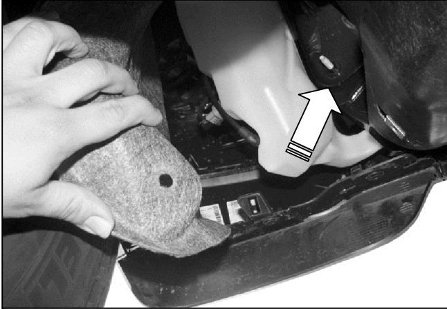
(Fig 9) 2014 model-reach up and in through gap behind bumper to reach and remove block-offs
