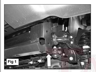
12mm x 25mm Hex Bolt 12mm Lock Washer 12mm Flat Washer
