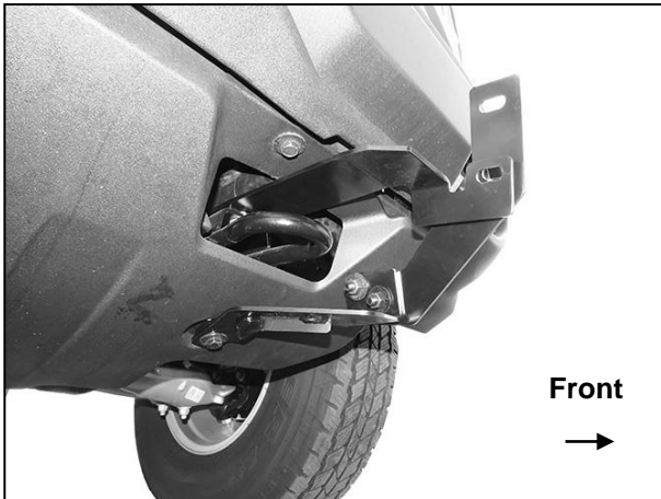
(Fig 11) Driver/left side Brackets installed
