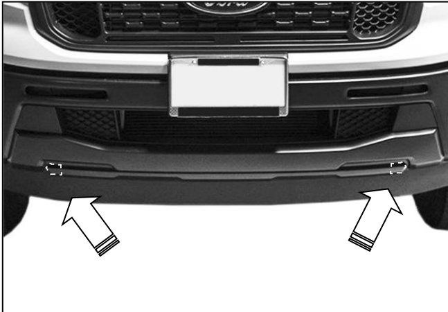
(Fig 5) Models without tow hooks, cut openings in lower plastic cover to clear Brackets
