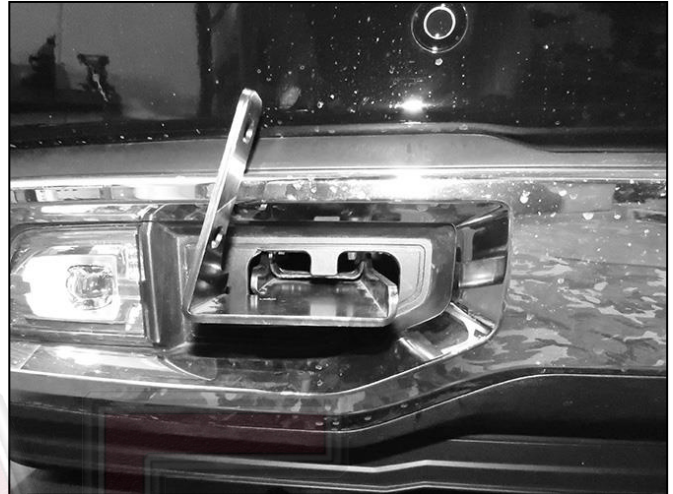
(Fig 11) Passenger/right side Bracket installed
