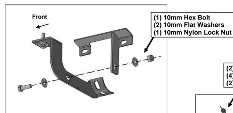
(Fig 3) Attach the Front Support Bracket to the <u>rear</u> side of the Front Mounting Bracket
