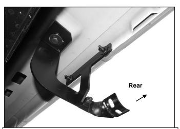
(Fig 7) Passenger/right side front Brackets installed
