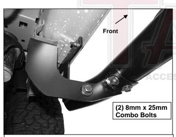
(Fig 17) Driver/left Sidebar attached to rear Bracket
