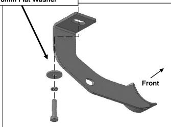
(Fig 3) Attach Driver/left front Mounting Bracket
