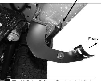
(Fig 14) Driver/left rear Brackets installed
