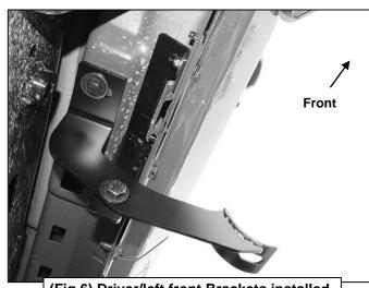
(Fig 6) Driver/left front Brackets installed
