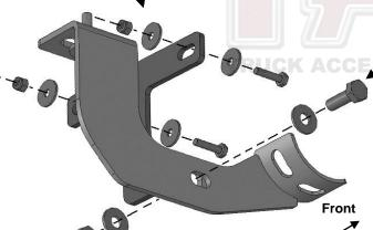
(Fig 13) Attach driver/left rear Support Bracket
