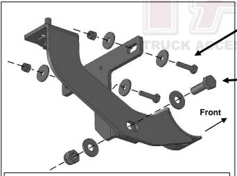
(Fig 9) Attach driver/left Center Support Bracket
