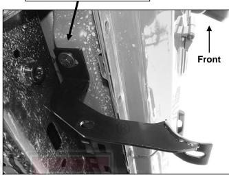
(Fig 4) Driver/left front Mounting Bracket installed
