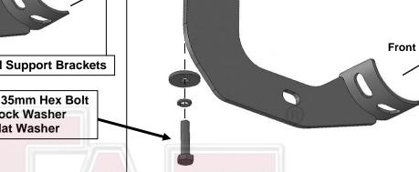
(Fig 12) Attach driver/left rear Mounting Bracket
