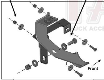
(Fig 5) Attach top of driver/left Support Bracket to <u>back</u> of pinch weld
