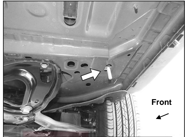
(Fig 17) Insert “Long” Bolt Plate into oval hole in front floor location (arrow)
