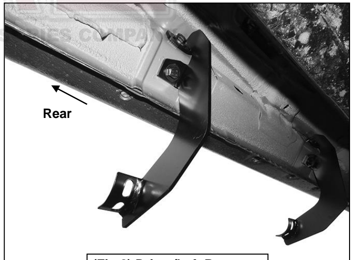
(Fig 8) Driver/Left Rear Mounting Bracket installed
