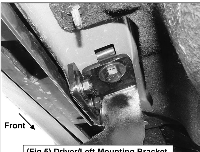
(Fig 5) Driver/Left Mounting Bracket attached to the front location
