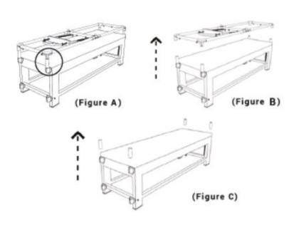
STEP 3 - PLACE THE VERTICAL PIPES AND CANOPY ON CADILLAC LOCATE THE ALLEN KEY AND 4 VERTICAL PIPES. LOOSEN THE SCREWS AND INSERT THE 4 VERTICAL PIPES INTO HE FLANGES ON THE CADILLAC FRAME. TIGHTEN THE SCREWS UNTIL THE VERTICAL PIPES ARE FIRMLY SECURE. CAREFULLY PLACE THE CANOPY ON THE TOP OF THE 4 VERTICAL PIPES (SEE FIGURE D). CAREFULLY TIGHTEN THE SCREWS UNTIL THE CANOPY IS FIRMLY SECURE ON TOP OF THE VERTICAL PIPES (SEE FIGURE E).
