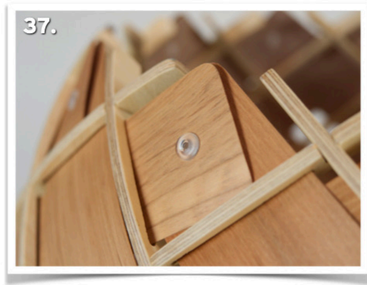
37. Apply pressure to one side of the rivet to help snap together. Listen for a 'click': One click good, two clicks best.
