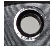
Bad (incomplete rounding)
