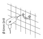
$\ensuremath{\mathbb{I}}$  . insert the wall plugs inside the holes
