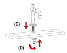
(C) Insert shank through center hole in sink.
