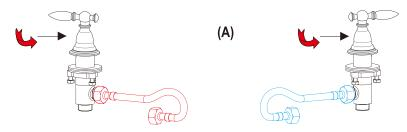
(A)Screw the handle body to the right until the handle off.
