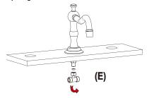
(E) Connect and tighten the T-Joint to the shank.
