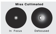
If the striped pattern can be seen as a concentric image, your telescope is properly collimated (aligned).
