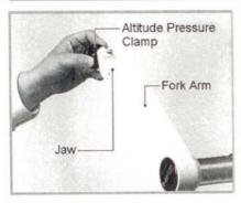
① Loosen the altitude pressure clamps and open the jaws of the upper side.
