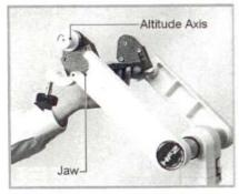
① Attach the swing bracket (optional) onto the lower jaws of the fork arms and cover the upper jaws. Tighten the altitude pressure clamps to hold it by friction.
