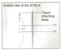
② Use one of the 1/4" screw holes on the bottom of the BT80-A to mount on the swing bracket.
