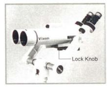
3 Tighten the lock knob firmly.
