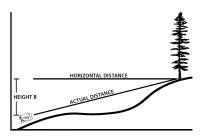
If you are standing at a level that is above the top of the object you are viewing, first point the rangefinder to the base of the object and obtain a measurement (Height A). Then point the rangefinder to the top of the object and obtain a measurement (Height B). Then subtract Height B from Height A to get the Height (A - B = Height).
