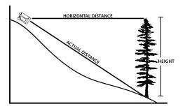
If you are standing at an elevation that is in between the top and bottom of the viewing subject first point the rangefinder to the top of the object and obtain a measurement (Height A). Then point the rangefinder to the base of the object and obtain a measurement (Height B). Then add those two numbers together to get the Height (A+B=Height).
