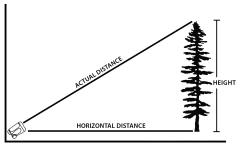
If you are standing level with the top of the object you are viewing, point the rangefinder to the base of the object and obtain a measurement. The Height will appear next to the word "High" in the LCD display.
