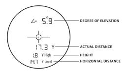
When viewing at steep inclines or declines, the actual distance to your subject is always longer than the horizontal distance. The horizontal distance takes into account the fact that your target might be at a different elevation than you are. Mode 2 displays both the actual and horizontal distances.
