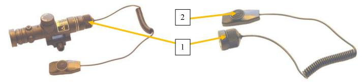
Now attach the Velcro pad onto the bottom (flat) side of the pressure pad. We suggest to attach Velcro the way where the soft side will be on the pressure pad and coarse side will stay on the weapon in order to prevent the weapon side to become dirty during exposure to outside elements.
