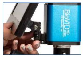
Remove the monitor from its packaging and mount the monitor to the camera's front mounting bracket using the included thumbscrew. Do not overtighten the thumbscrew but ensure you securely tighten it to prevent the monitor from falling off of the camera.
