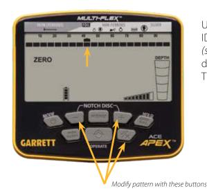
Use the NOTCH DISC buttons to position the Target ID Cursor above the pixel you wish to eliminate (see illustration to left). Use the ( $\checkmark$ /x) elim button to delete this pixel from the Lower Scale (see below). This item is now rejected.
