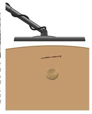
Therefore, the gold coin is detected due to the combined conductivity being higher than that of the discriminated target (nail) alone.
