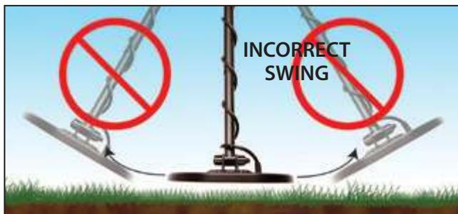
Swing your searchcoil parallel to plow lines and the water's edge. This will minimize the negative effects caused by uneven ground in plowed fields and varying amounts of moisture near the water. Do not swing the searchcoil perpendicular to plow lines and the water's edge, as this may produce abrupt changes in ground response that can reduce the detector's performance.
