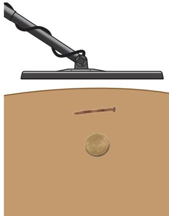
Therefore, the gold coin is detected due to the combined conductivity being higher than that of the discriminated target (nail) alone.
