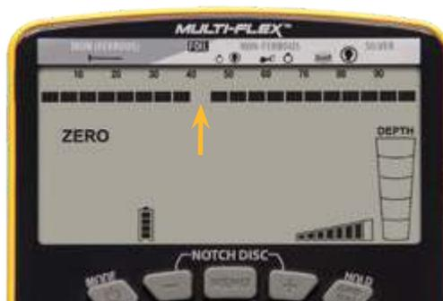
Use the NOTCH DISC buttons to position the Target ID Cursor above the pixel you wish to eliminate (see illustration to left). Use the (✓/x) elim button to delete this pixel from the Lower Scale (see below). This item is now rejected.
