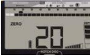
In this illustration, Apex is operating in Zero Mode with two pixels of iron eliminated. This nail registers from 18 to 24 on the Digital Target ID scale. To eliminate the nail from detection, notch three more pixels of iron.
