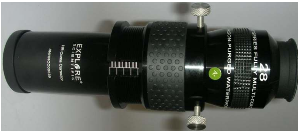
Figure 4: HR Coma Corrector with eyepiece that has a field stop 3mm below reference
