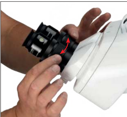
17. Focusing by means of helical single focusing.
