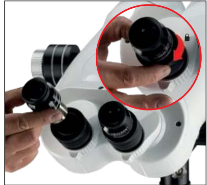
16. Insert and clamp the eyepieces.
