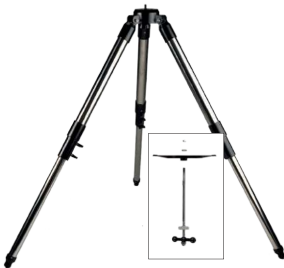
Tripod with spacing plate and central screw
