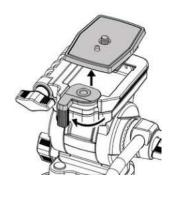
Insert mounting screw into thread on optic and turn wingnut (located on underside of quick release plate) clockwise until tight. This will secure optic to plate.
