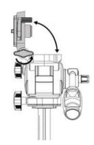
4. To adjust pan/tilt handle angle, loosen locking knob by turning counter clockwise until interlocking teeth disengage. Position handle as desired and tighten knob to lock.
