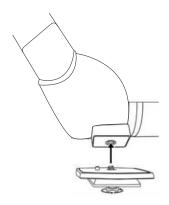
3. Reattach quick release plate to tripod head. Press down plate and lever will shift into place and lock.
