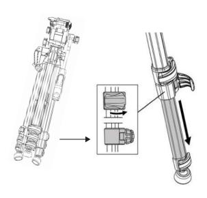
2. Loosen center column locking collar. Spread tripod legs to desired width. Tighten collar to lock in place.
