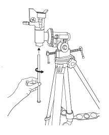
6. Screw the Counterweight Bar into Counterweight Threaded Hole on Equatorial Mount.
