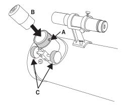
16. Loosen thumbscrew on Focuser Draw Tube (A). Slide Eyepiece (B) into Draw Tube and tighten thumbscrew (A). Finding targets will be easier if you start with K20 Eyepiece. Adjust Focus Knobs (C) until image is clear.
