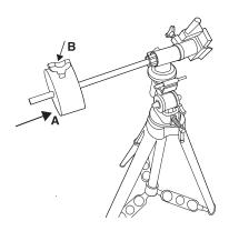
8. Slide Counterweight (A) a quarter of the way up Counterweight Bar. Tighten Counterweight Knob (B) securely. See video tutorial for proper balancing at carson.com/mytelescope Warning: If counterweight is not secured (fully tightened with counterweight knob at balance point), the telescope can become unstable and tip over.
