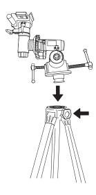
Loosen Tripod Knob. Attach Equatorial Mount to Tripod and tighten with Tripod Knob.
