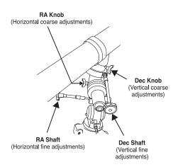
To position Optical Tube to desired angle, adjust RA/Dec Knobs. Use RA/Dec Shafts to fine-tune OTA if necessary.
