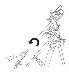
Use a Phillips Screwdriver to remove the Safety Screw and Washer on the Counterweight Bar.
