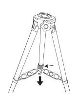
Extend **Tripod** legs to widest position. Gently push down tripod braces and tighten lock knob.
