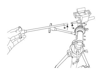
11. Remove rubber cap on Dec Shaft (A). Loosen thumbscrew (B) on Slow Motion Cable and slide onto Dec Shaft. Tighten thumbscrew (B) to flat notch on shaft.
