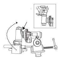
3. Loosen the **Right Ascension Knob** on **Equatorial Mount** to flip mount upright. Tighten **Knob** to secure.
