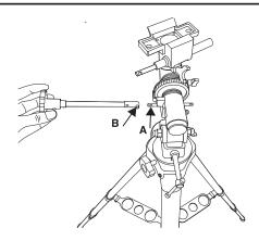
10. Remove rubber cap on RA Shaft (A). Loosen thumbscrew (B) on Slow Motion Cable and slide onto RA Shaft. Tighten thumbscrew (B) to flat notch on shaft. Note: Cable can be placed on either side of mount.
