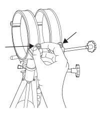
13. Loosen and remove thumbscrews on each **Cradle Ring.**
