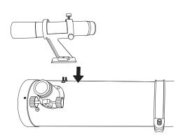
15. To attach **Finderscope**, remove **Thumbscrews** on OTA and place Finderschope onto mounting screws. Reattach thumbscrews and tighten to secure.
