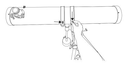
14. Open Cradle Rings and insert OTA. Cradle Rings should be in the center of the OTA. Close Rings and tighten thumbscrews to secure OTA with cradle rings. For proper balancing, the Focuser Draw Tube should be facing upwards and Focuser Draw Tube and Counterweight should both be on same side of tripod. See video tutorial for proper balancing at carson.com/mytelescope
