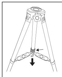
Extend **Tripod** legs to widest position. Gently push down tripod braces and tighten lock knob.
