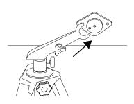
5. Slide **Alt-Az Arms** behind mounting brackets on each side of tube. Tighten screws to secure.
