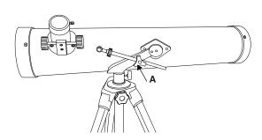
Loosen Vertical Adjustment Knob (A) to allow Altitude Rod to slide through and connect to threaded hole on Alt-Az Mount Arm (B). Use the included Slotted Screwdriver to attach Altitude Rod Screw to the OTA Threaded Hole.
