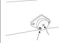
4. Using a Phillips Screwdriver, loosen both screws on both **OTA Mounting Brackets.**
