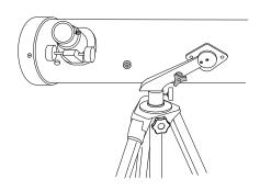
Note: OTA Threaded Hole and Vertical Adjustment Knob should be on same side of OTA.
