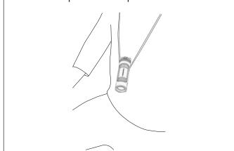
1. To reduce glare, twist eyecup into outermost position. If you wear eyeglasses, you can twist eyecup down to improve field of view.
