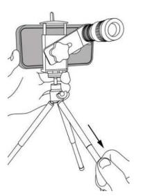
Extend each tripod leg out fully to increase stability.
