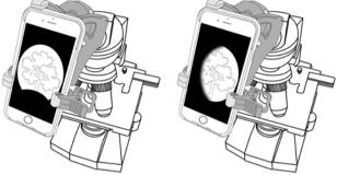
**A6:** The phone alignment needs to be adjusted in vertical direction using top clamp (FIG 7) and in horizontal direction by using alignment screw (FIG 8). Check that phone is flat on adapter (FIG 6), and adapter is flush with optic.
