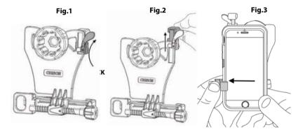
Rotate to unlock top clamp.
