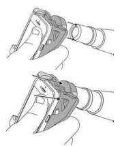
Align optic adapter over eyepiece and press down firmly. Be careful not to move your camera out of alignment.
