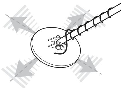
*When pinpointing a target, try drawing an "X", as illustrated, over where the tone is induced.*
