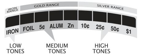
The faceplate label is color-coded above the Conductivity Arc. Ferrous, gold and silver targets will generally register within their corresponding color-coded ranges. Targets that are not gold or silver register within the same range according to their electrical conductivity.
