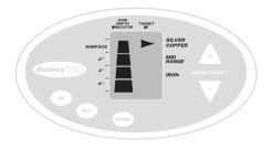
More deeply buried objects will illuminate more segments, indicating depths of 2, 4, or 6 inches, as identified to the left of the display. The depth indicator is not accurate for large, or irregularly shaped, objects.
