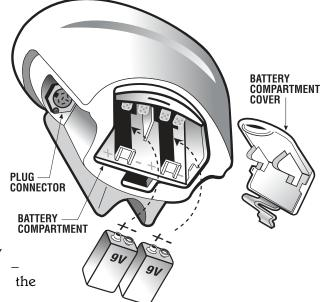
3 Insert (2) 9-Volt **ALKALINE** batteries, with the contacts pointed inward, and press down on the back of the batteries to snap them into place.
