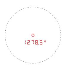
b. Tilt Angle mode (T): Aim the reticle at a target. Press the button once to measure the distance. The linear distance of ranging is displayed first (1). After 1 second, Angle value is displayed (2). After another second, display returns the linear distance of ranging (3).
