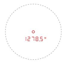
b. Golf Mode: In a group of targets, hold the ① button while aiming at the target for scanning. The nearest target is locked first. The values displayed on the screen do not change (nearest distance).
