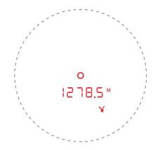
4. DISPLAY BRIGHTNESS ADJUSTMENT: Short press button to select between level 1 to 4 display brightness. Press button to confirm the item you selected or skip this option and return to ranging.
