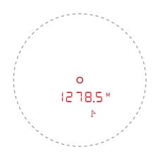
c. Hunting Mode: In a group of targets, hold the button while aiming at the target for scanning. The farthest target is locked first. The values displayed on the screen do not change (farthest distance).
