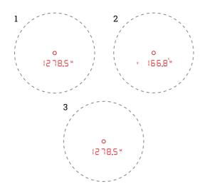
d. Horizontal Distance mode: Aim the reticle at a target. Press the button once to measure the distance. The linear distance of ranging is displayed first (1). After 1 second, the Horizontal Distance is displayed (2). After another second, display returns the linear distance of ranging (3).
