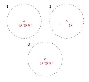
c. Vertical Distance mode (V): Aim the reticle at a target. Press the button once to measure the distance. The linear distance of ranging is displayed first (1). After 1 second, the Vertical Distance is displayed (2). After another second, display returns the linear distance of ranging (3).
