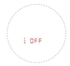
a. LOS mode (OFF): Aim the reticle at the target. Short press log button once to measure the distance. Only the linear distance of the ranging is displayed.
