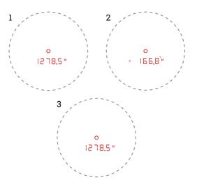
3. MEASURING METHOD SELECTION: "Auto", "Flag", "Deer" will start blinking. Short press 🕑 button to select "Auto" for Regular Mode, "Flag" for Golf Mode, or "Deer" for Hunting Mode. a. Regular Mode: In Regular Mode hold (2) button while aiming at the target for scanning. The distance value on the screen varies with the target.
