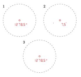
c. Vertical Distance mode (V): Aim the reticle at a target. Press the 🕜 button once to measure the distance. The linear distance of ranging is displayed first (1). After 1 second, the Vertical Distance is displayed (2). After another second, display returns the linear distance of ranging (3).
