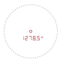
**b. Tilt Angle mode (T):** Aim the reticle at a target. Press the O button once to measure the distance. The linear distance of ranging is displayed first (1). After 1 second, Angle value is displayed (2). After another second, display returns the linear distance of ranging (3).
