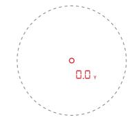
2. Menu select: Long press is button for 2 seconds to enter the mode setting menu. Using the is button you can scroll through the icons. Short press is button to advance to the next screen. In mode setting menu long press is button for 2 seconds to return to ranging display.
