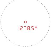
**b.** Golf Mode: In a group of targets, hold the **b** button while aiming at the target for scanning. The nearest target is locked first. The values displayed on the screen do not change (nearest distance).
