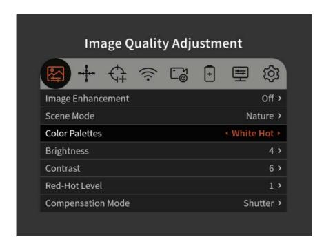
**Brightness:** Detector brightness can be adjusted within 1-10 levels.
