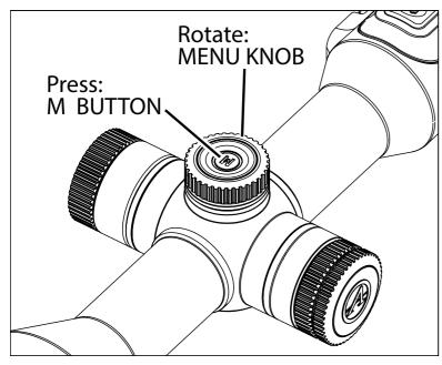
When the scope is powered on for the first time to select the language, rotate the "Menu Knob" to scroll up and down to select the language; Short press the "M Button" to confirm the language selection and jump to the Home interface; long press The "M Button" to return to the language scrolling selection.
