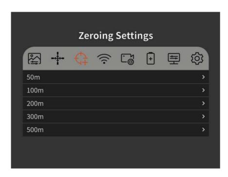
One Shot Zeroing: Prior to using the one shot zero function, you must set the Zeroing Distance by accessing the short menu.
