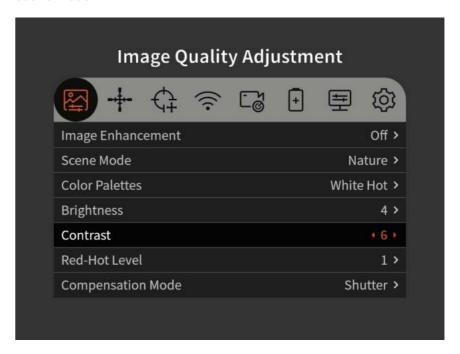
**Red Hot Level:** Red hot level can be adjusted within 1-10 levels.
