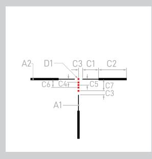
The MOA #05 reticle is a bullet drop compensation reticle specifically designed for 5.56 mm NATO /.223 REM round. The holdovers for bullet drop are extended to 200, 300, 400, 500, and 600 yards.
