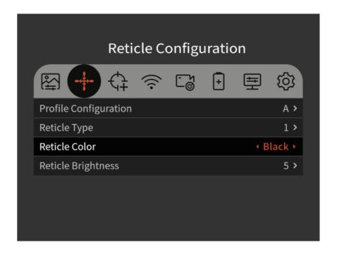
**Reticle BRI:** Reticle BRI can be adjusted within 1-10 levels.
