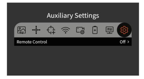
**Remote Control:** After being turned on, it will search for Bluetooth remote control connection. After successful connection, all functions of the button on the scope can be controlled by the Bluetooth remote control (except the function required by long press). The bluetooth remote has 1 hardware switch and 4 buttons. Among them, the hardware switch controls the on and off of the remote control itself. The 4 buttons correspond to the 4 buttons on the scope as shown in the figure below
