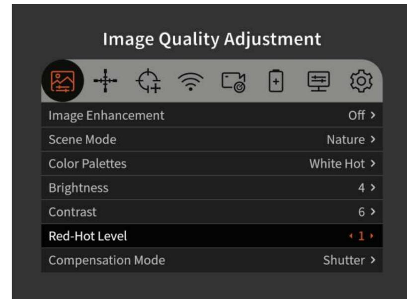
**Compensation Mode:** Scene/Shutter Mode can be set through the Main Menu. Scene Mode sets short pressing the power button to capture an even temperature surface to refresh the thermal sensor. The best way to perform Scene Mode compensation is doing it with the lens cap closed. Shutter Mode sets short pressing the power button to close the device shutter and create an even temperature surface to refresh the thermal sensor.
