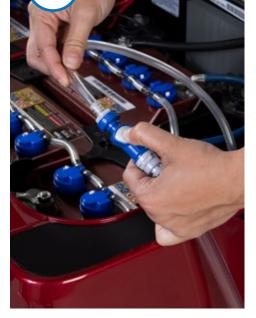
Always disconnect the pump after watering.
