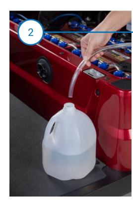
Insert the open end of the pump into a jug of distilled water.
