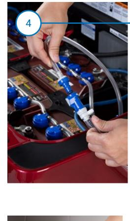
on the watering system into the female connector on the manual pump.
