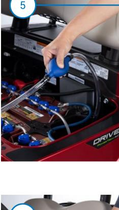
Squeeze the bulb on the manual pump to begin filling the battery cells with water.
