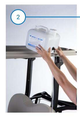
Tank should be positioned 3 feet or more above the batteries to ensure proper water flow.
