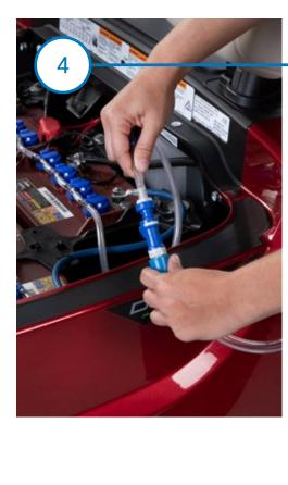
Connect by inserting the male connector on the watering system into the female connector on the gravity tank fill line.
